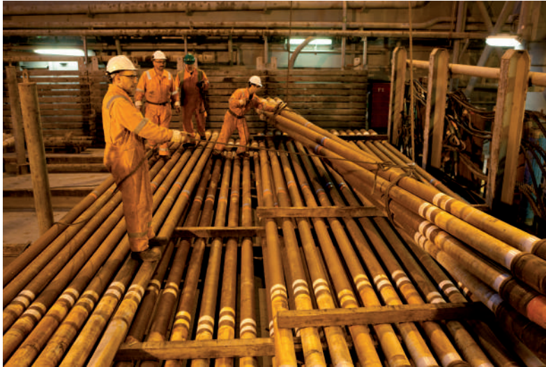
Arrival of drill strings at the ADB 001 Absheron platform.
